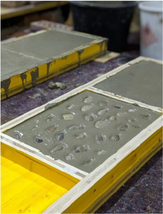
I River stones placed on the not-yet dry concrete
