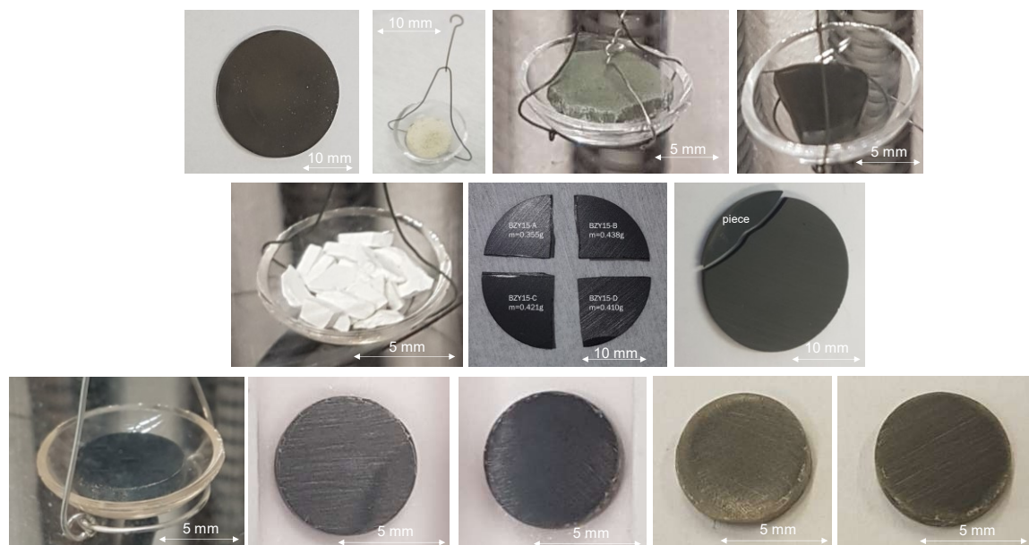
Figure 14: Images of all samples (First row: BZCY81-TGA1, BZY15-Powder, BZY15-TGA2, BZCY81-TGA3 second row: BZY15 pieces, BZY15 Pellet 1, BZY15 Pellet 2 third row: In-house sintered BZY15 Pellet 1, 2, 3, 4 and 5)
