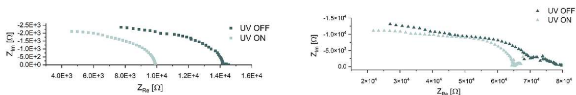
Figure 4.19: Exemplary impedance measurements of PK006 and PK007 at 300°C in the dark and under UV light irradiation. Left: PK006 contacted at the down left electrode. Right: PK007 contacted at the up right electrode.
