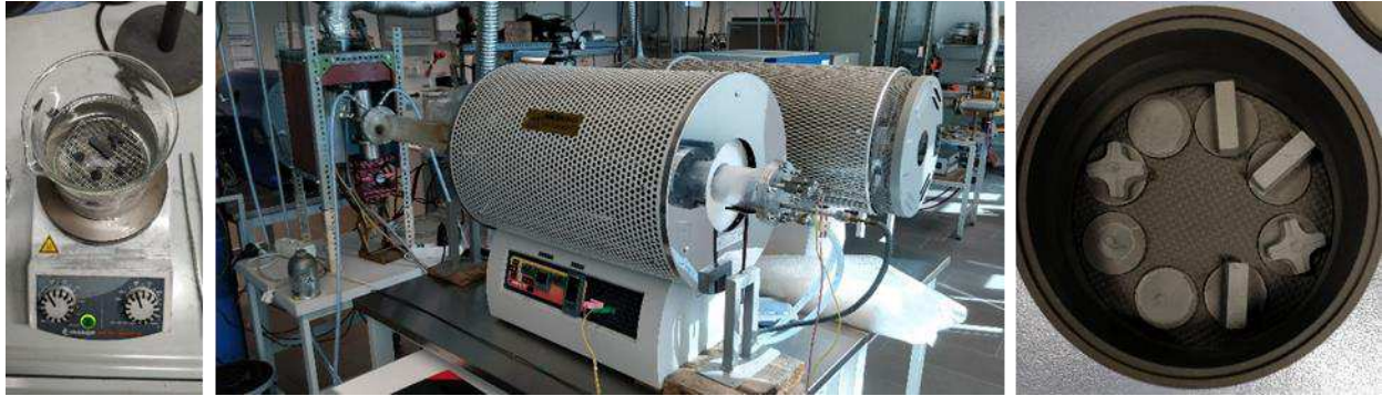
Fig. 8 From left to right: Beaker with samples in Cyclohexane, tube furnace for thermal debinding, graphite crucible with arranged samples
