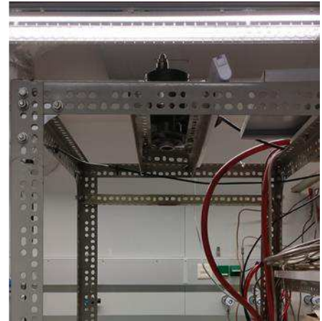
Fig. 10 Left: sintering profile recommended by Hyperion, right: infrared pyrometer on top of the furnace
