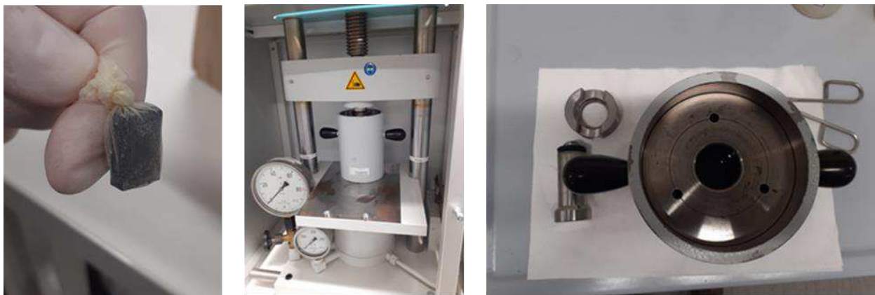
Fig. 12 From left to right: Sample packed in a latex bag ready for CIP, uniaxial press, compression mould (Paul-Otto Weber GmbH)
