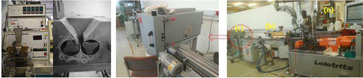
Fig. 4 From left to right: Kneader for preliminary tests, pelletizer, twin screw extruder with conveyor belt – pictures provided by Mr. Duretek (MU Leoben)
