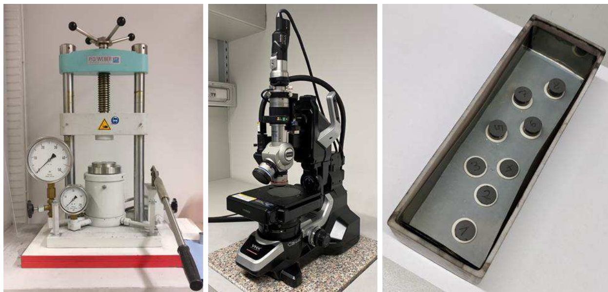
Fig. 11 From left to right: uniaxial press, digital microscope, pressed samples on \text{Al}_2\text{O}_3 support plate ready for thermal debinding
