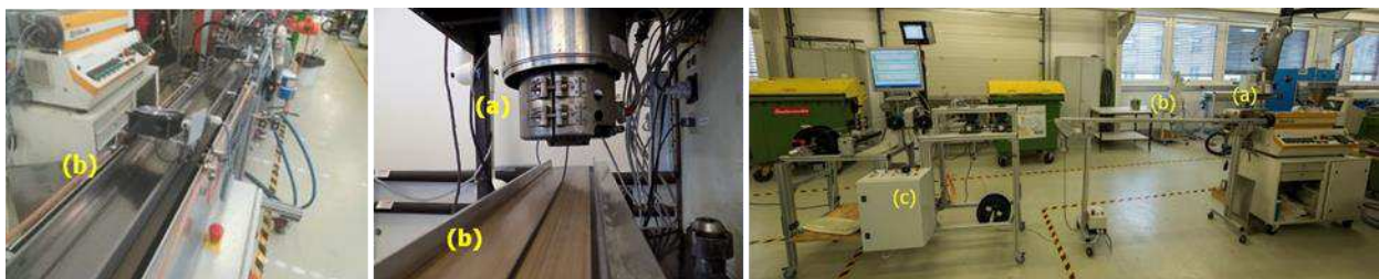
Fig. 5 From left to right: metallic conveyor belt from 3.4 Production of the feedstock, capillary rheometer with Teflon conveyor belt, filter-test-extruder with haul off and winding unit – pictures provided by Mr. Duretek (MU Leoben)
