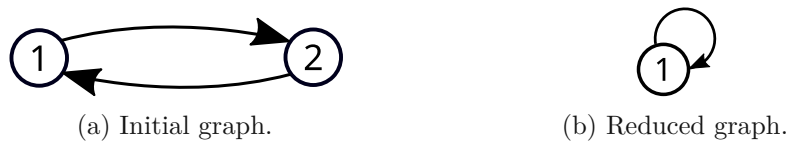
Figure 4.5: An example of how self-loops can be introduced by the reduction rules. When applying, for example, rule IN1 to vertex 2 in the initial graph, then vertex 1 ends up with a self-loop in the reduced graph.
