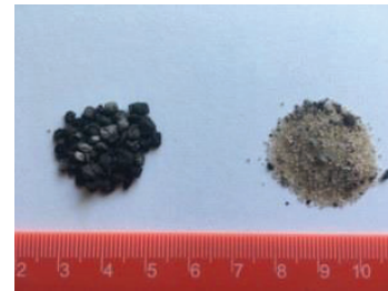
Fig. 5: Coherent ash particles from combustion of lignin in the FB reactor
