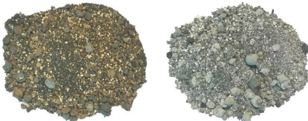
Fig.8: Bed material ash mixture from the combustion reactor entering the gasification reactor (left: brown-red colored) and leaving the gasification reactor (right: gray colored)
