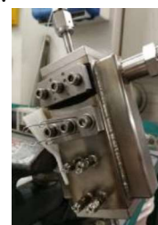
Manufactured millistructured reactor (mini scale)
