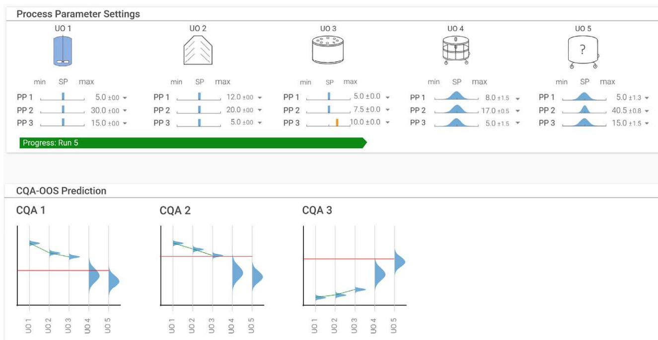
Figure 7. Proposed control panel for IPM use in a real-time environment. Process parameters may be controlled manually or through targeted APIs to either create a prediction around the process parameter (set point plus expected normal operating variation) or to bring in the discrete value when the PP setting is known. Predictions via MC simulations around the chance of specification conformity can be updated immediately. Refitting the models may also be performed in real time or at regular intervals.
