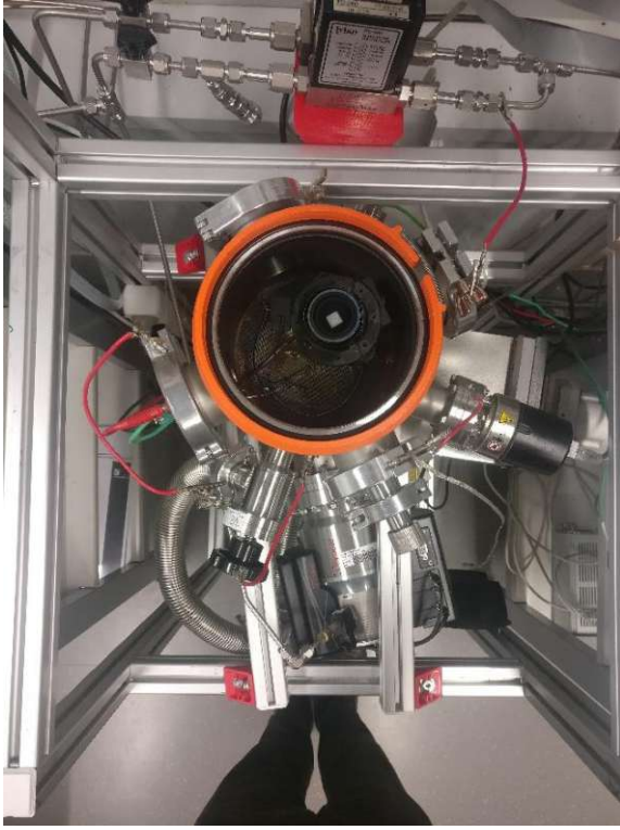
Figure 44: Top view of the sample chamber.
