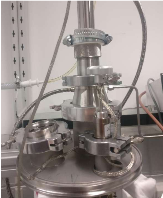
Figure 42: Detail of the top flange, showing a window, the gun feed through as well as the mechanical feed through for turning the shutter inside.
