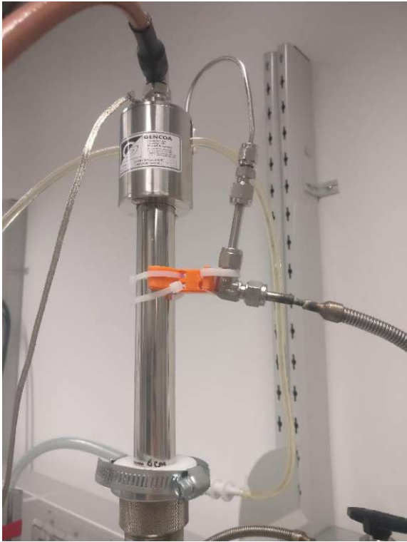
Figure 40: Top of the shaft of the sputter gun, fed through the top flange. Clear polymer tubing for water cooling, stainless steel gas tubing and the electric connection to the RF-Power supply (brown cable) are visible.
