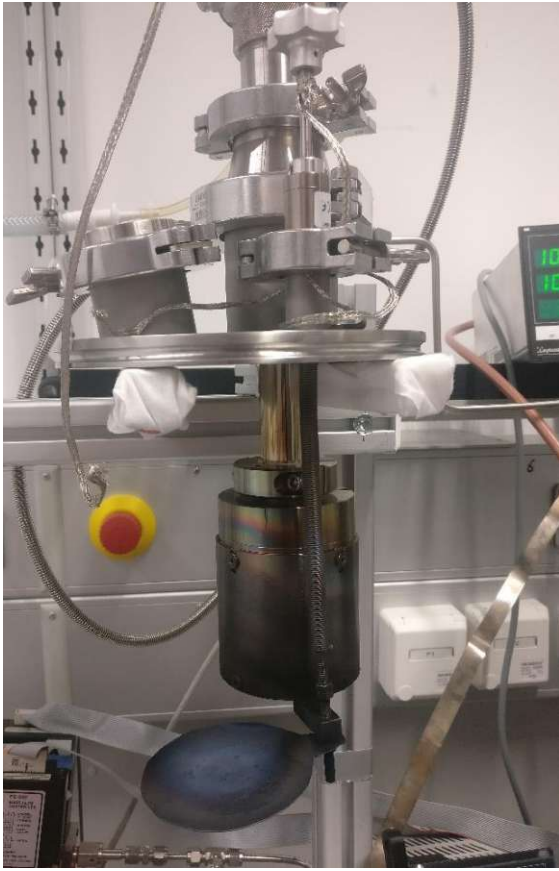
Figure 43: Top flange and sputter gun with opened shutter.
