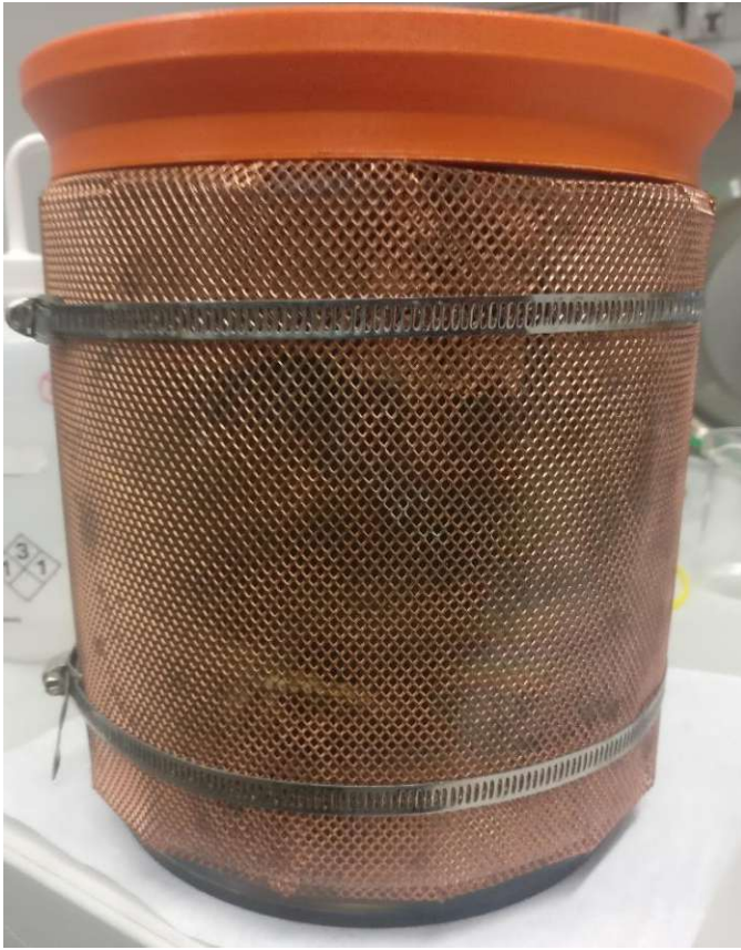
Figure 36: Glass recipient, surrounded by a polymer safety shield and a copper mesh for electric shielding.
