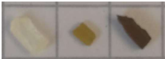
Figure 26: Pristine LLZO (left), sample after annealing with a LCO thin film on top and parts of LLZO removed (middle), and with annealed LCO thin film (right).
