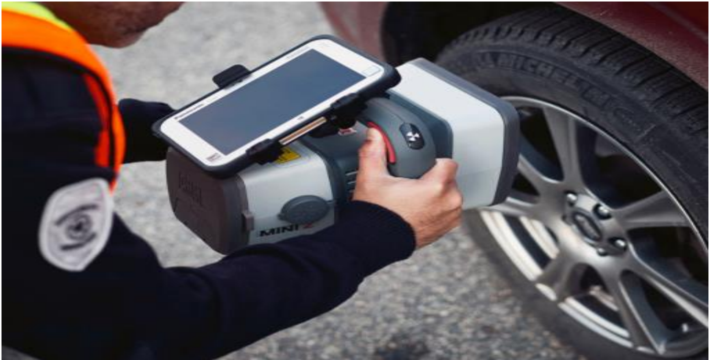
Picture 16: Customs Officer uses handheld device based on Z Backscatter technology (MINI Z) when inspecting vehicle for contraband drugs and currency. Source Rapiscan Systems and AS&E.
