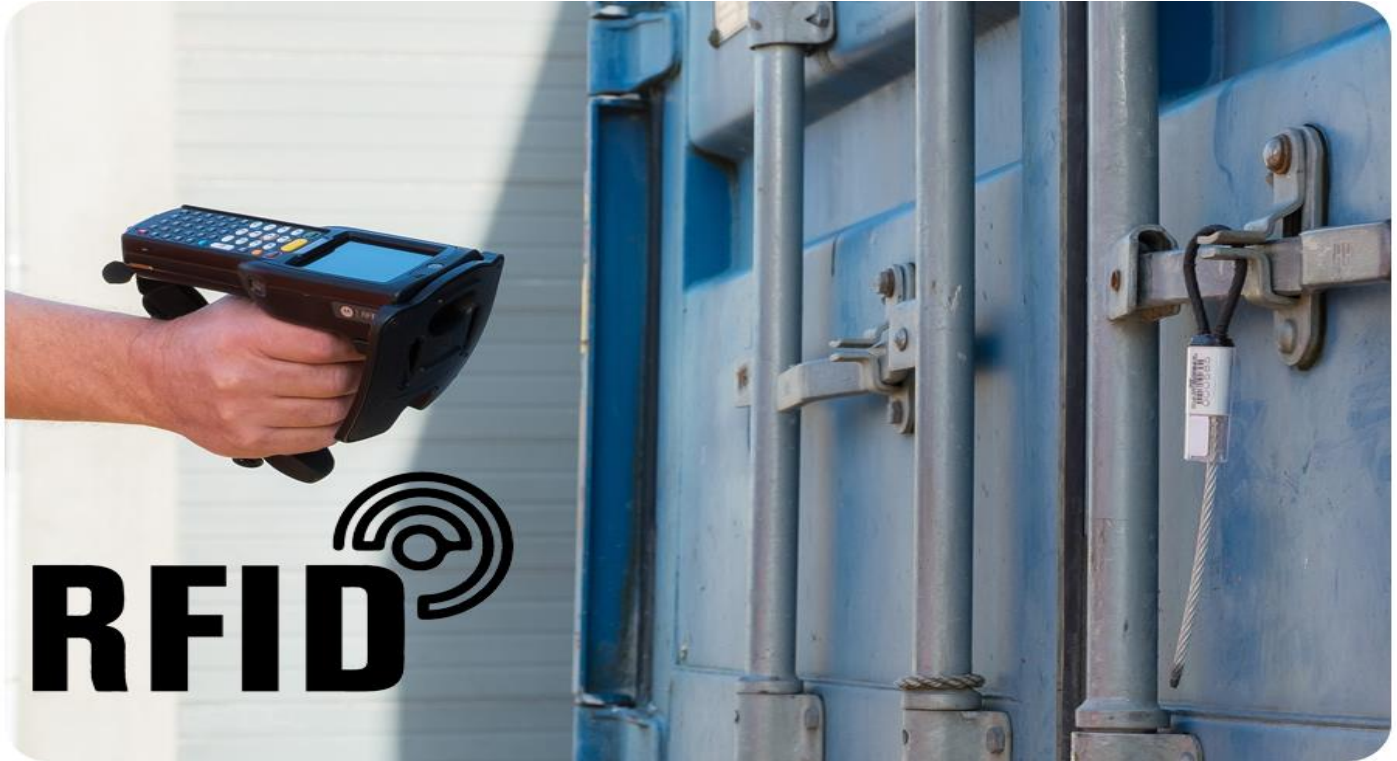
Picture 7: RFID Handheld Reader to read RFID E-Seal at Customs Station. Source Harcor, www.harcor.com.
