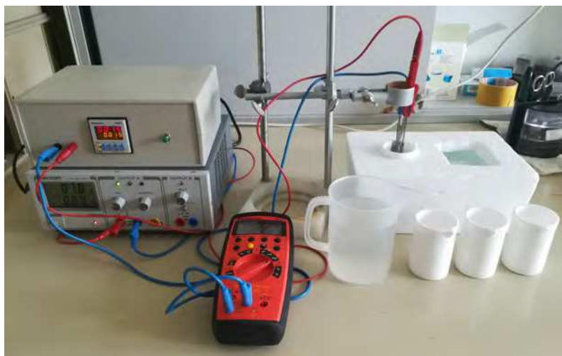
Figure 2.11: Flash electro-polishing setup.
