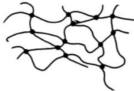
Fig. 1.6: The chain molecules of a thermoset are closer bonded and have got a higher cross-link density than an elastomer. Those chains are not able to move against each other under a thermal load [45].
