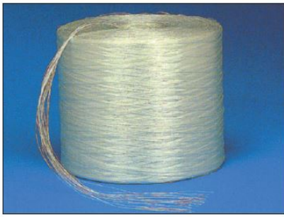
Fig. 1.10: Continuous glassfibres assembled to rovings and spooled on a bobbin [46]
