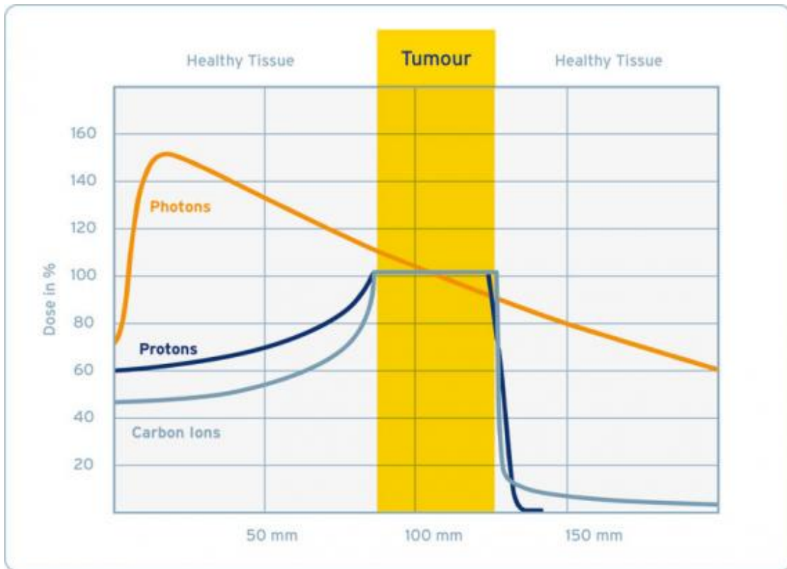
Figure 2.1.: Percentage Depth Dose Curves for Photons, Protons and Carbons. Proton and Carbon Curves are shown with a spread-out Bragg Peak, Photons as a Single Energy Beam [6]
