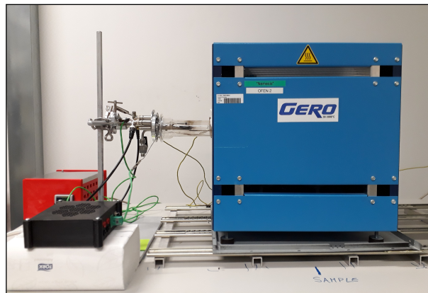
Figure 3.4: Measurement setup for impedance measurements
