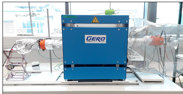
Figure 3.7: Measurement setup for voltage measurements under UV light irradiation
