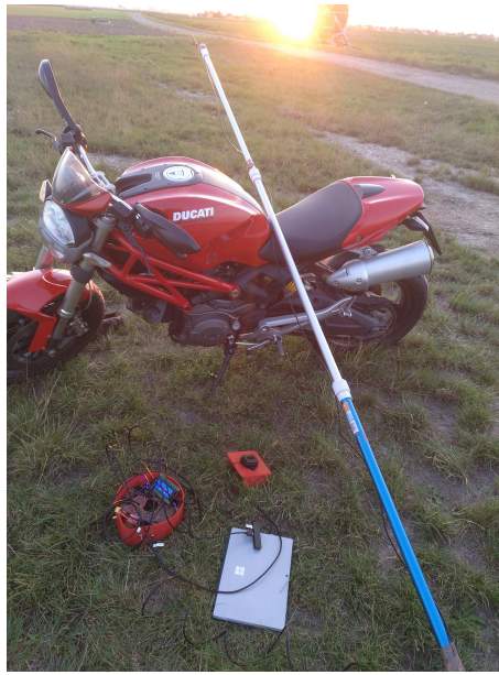
Figure 4.35: Rover with LoRa antenna on a 3.6 m rod.
