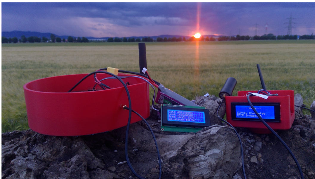
Figure 4.26: RTK system working at the dynamic measurement place.
