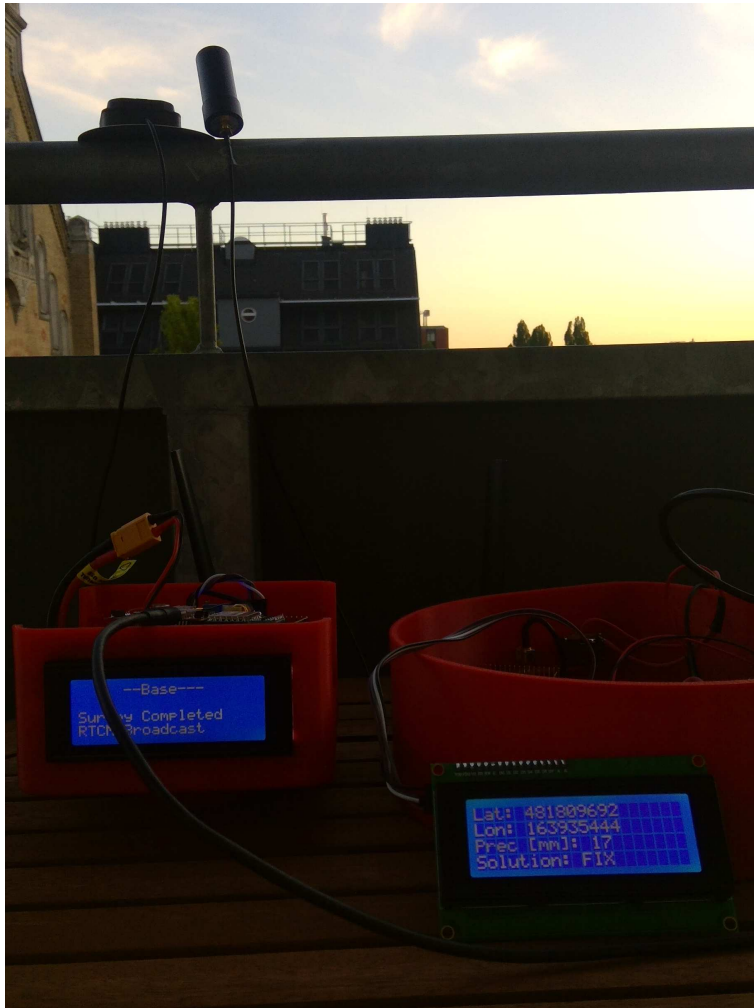
Figure 4.6: RS (left) and rover (right) during static RTK-measurements.
