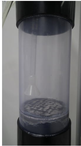
Figure 12: Picture of the column including the distribution plate and the riser
