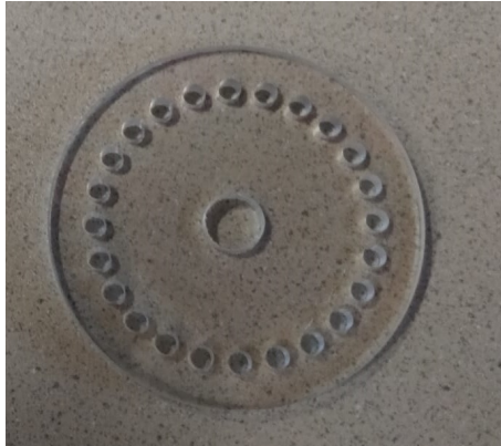
Figure 29: Picture of the perforated disc used in the Revolver Doser (RD).
