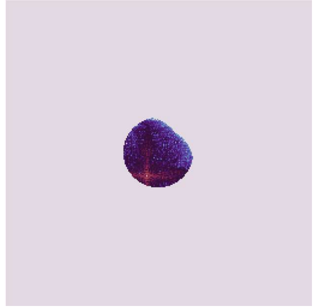
Figure 2.5: Magnitude of the spectrum of low-resolution complex object \hat{o} during the first loop of FPM recovery. The size of the disc corresponds with the cutoff frequency \pm k_{co} .
