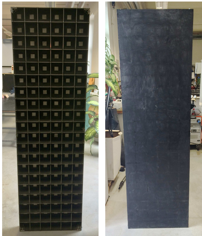
Figure 5.16.: Absorber array consisting of 120 mass loaded membranes on a 80 mm deep rigid steel frame.
