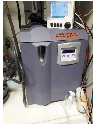
Figure 10 Principle scheme (left) and photo (right) of the proton exchange membrane (PEM) electrolysis
