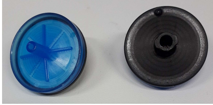
Figure 17 Syringe attachment filters, two steps 180 \mu m and 0.45 \mu m pore wide (CHROMAFIL GF/RC-45/25)
