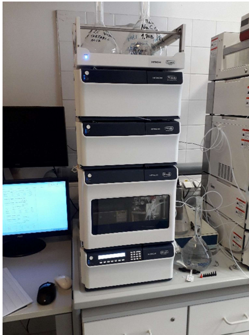
Figure 16 High performance liquid chromatography HITACHI Primaid, including Aminex HPX-87 H column and UV-Detector
