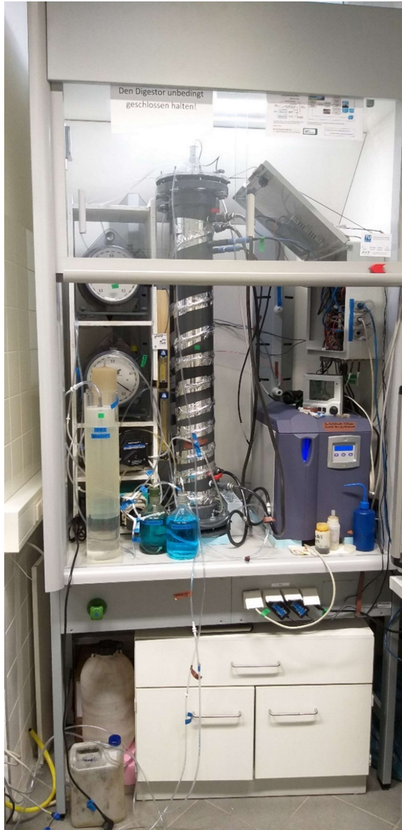
Figure 8 Experimental installation with the hydrogen generator and the gas collector (picture on the left). Reactors with connection tubes, probes, heating mantel and stirring drive (picture on the right).
