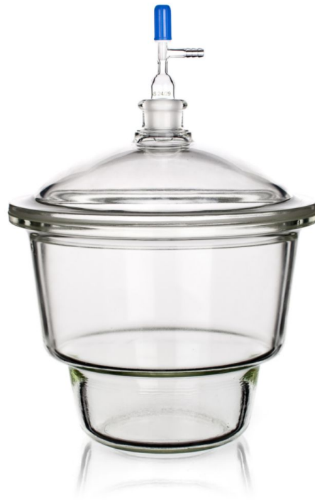
Figure 3.2.: Low Vacuum Glass Desiccator [71] used to dry out collagen fibrils on microscope slides at multiple points in the experimental process before and between measurements. The vacuum is applied at the upper valve by an external vacuum pump.
