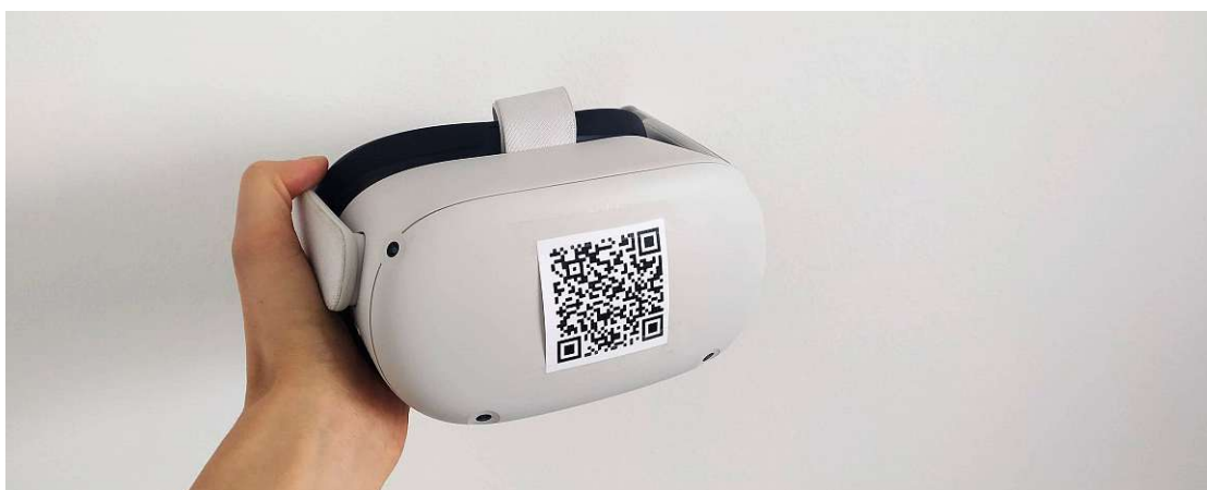
Figure 4.2: The setup of the HMD with the QR-Code.
