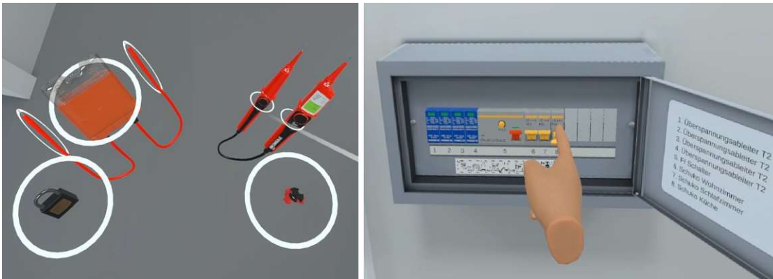
Figure 4.4: Voltage tester, test lamp and two locks (left) and the fuse box in the hallway (right).
