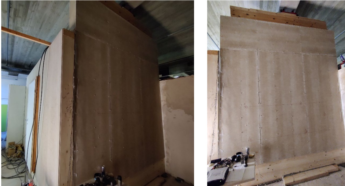
Figure 4 - T-joint and closed receiving room
