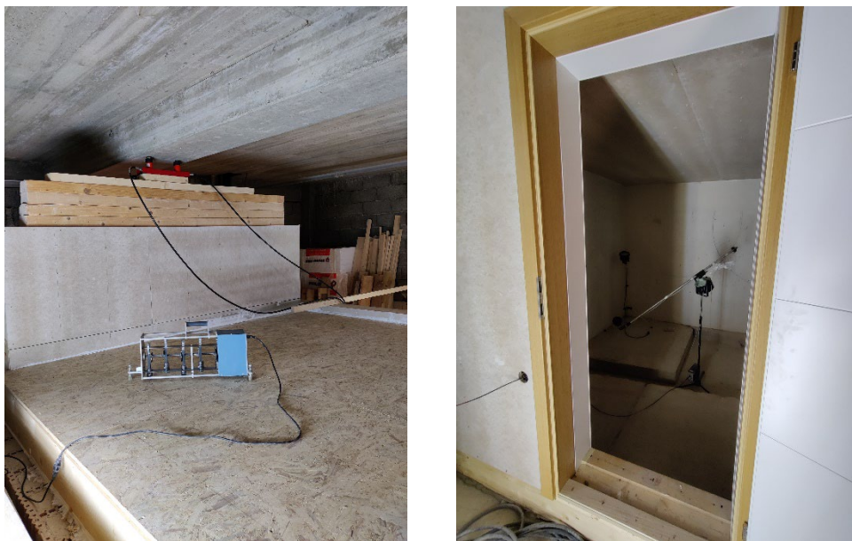
Figure 2 - (Left) Tapping machine on the wooden frame ceiling; (Right) Rotary boom microphone for sound pressure level measurement in the receiving room
