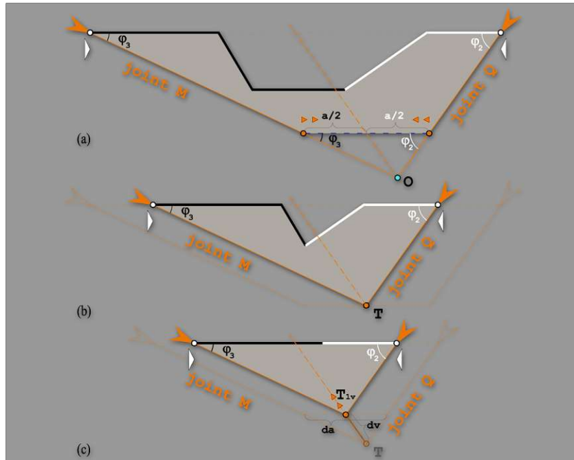
Figure 7.9: Contraction of the feature collection beyond length zero. (a) shows a situation somewhere along the corner side; (b) shows the situation when the base line reaches the top \mathbf{T} and becomes zero (i.e. a point); (c) shows the next contraction step: the effect is that the intersection point of the joint lines moves away from the point in (b). Figure 7.10 shows the symmetrical case and Figure 7.12 - the asymmetrical case in 3D.
