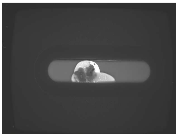
Figure 39: CN150W membrane with glued on powder in Prototype 3; Bright areas correspond to bare glue, dark areas to glued-on powder. t_{int} = 10 ms, cassette used = ABSW
