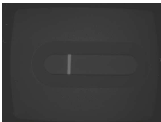
Figure 24: Reference membrane, image taken with optical longpass filter GG475; t_{int} = 10 ms, cassette used = ABSW
