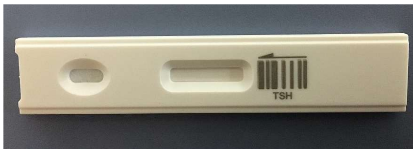
Figure 40: AllTest TSH test strip; samples are applied in the sample application window on the left side, the read-out window is located in the middle of the test strip cassette.
