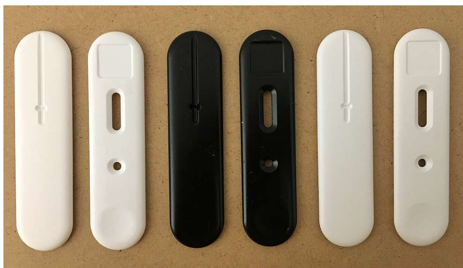
Figure 21: Tested cassettes, from left to right: white ABS, black ABS, white Makrolon; dimensions in assembled state: 105×27×6 mm
