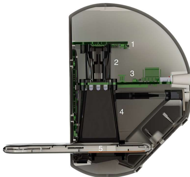
Figure 13: Inner side view of the Bloom Lab; CMOS sensor PCB (1), upper lightcone (2), main PCB (3) with LEDs, lower lightcone (4), test cassette inlet (5); total height = 121.6 mm
