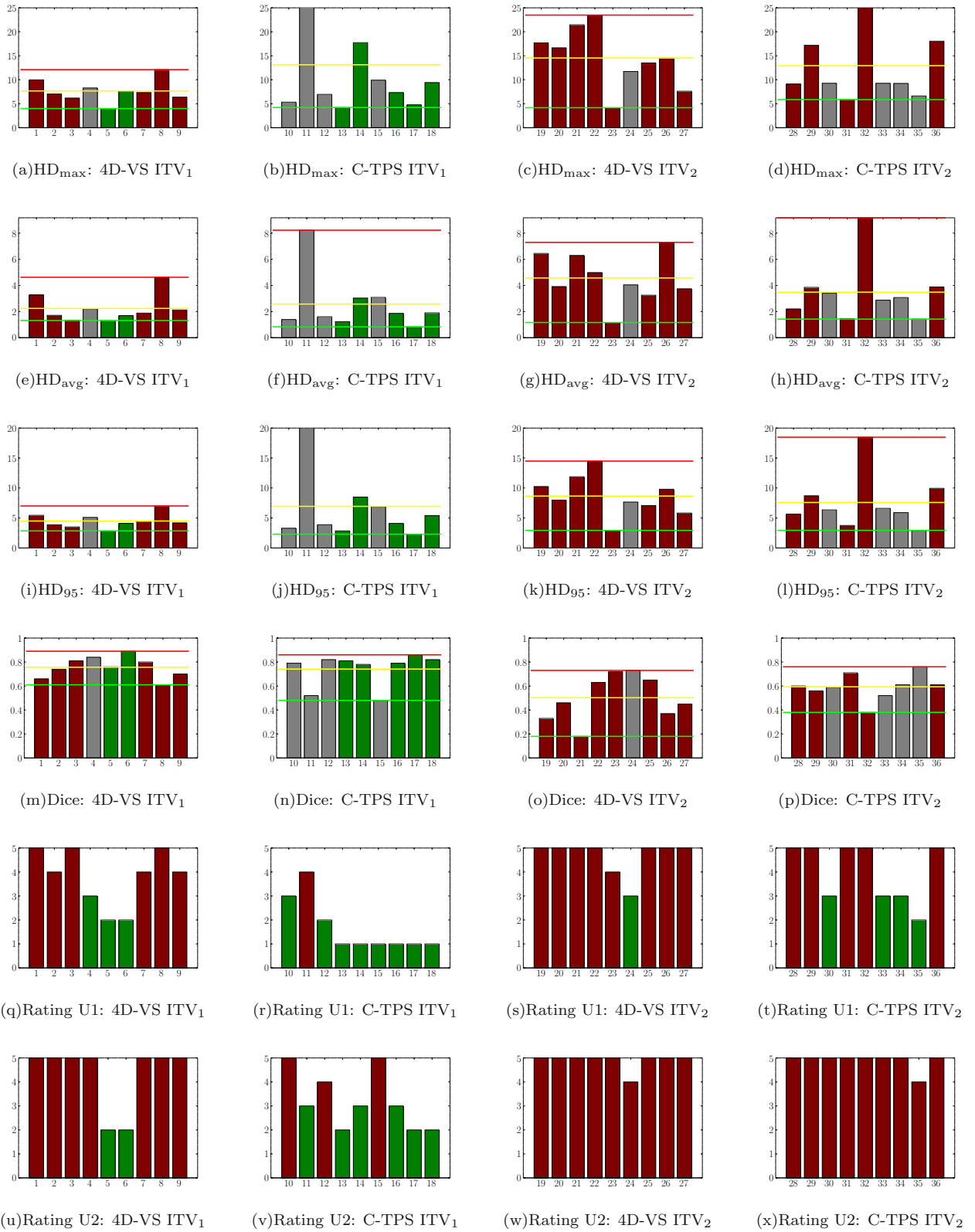
FIG. 1. Graphical overview of individual test cases used in Task T.1. Columns represent results for 4D-VS ITV 1 , C-TPS ITV 1 , 4D-VS ITV 2 and C-TPS ITV 2 (in that order). The first four rows represent the quality measures used to compare ITVs to the planning ITV. From row one to row four these measures are: maximum ( HD_{\max} ), average ( HD_{\text{avg}} ), 95% ( HD_{95} ) Hausdorff distance and the dice coefficient. They also have lines for the minimum (green), average (yellow) and maximum (red) values within one subplot. For plots where the maximum value lines were omitted, the maximum value was cropped to the highest displayed y-coordinate (see Tables I–IV for the exact value). The last two rows represent the user ratings for U1 and U2. The bar colors were chosen as follows. Green bar represents an accepted case, a red bar represents a rejected case, and a gray bar (does not apply to user ratings) represents a case, which was rejected by one user and accepted by the other.
