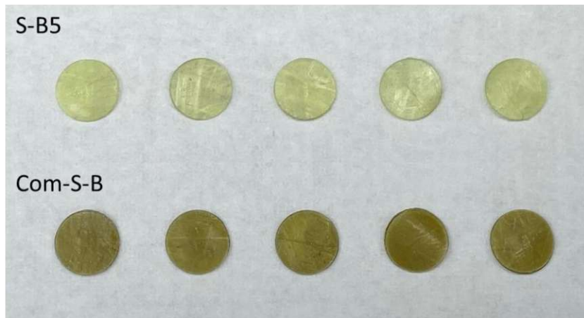
Figure 198: BADGE-based discs fabricated via hot lithography by the use of initiator S-B5 and Com-S-B (photographed around 10 h after printing)
