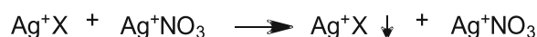
Figure 64: Precipitation reaction of a positive halogen test ( A^+ ...onium ion; X^- ...halogen counter ion (Cl - , Br - , I - ))
