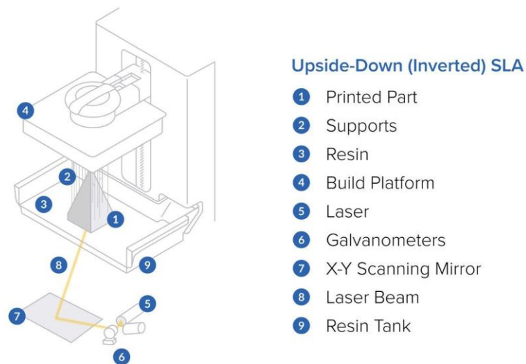
Figure 3: Scheme of a stereolithography 3D-printer 13
