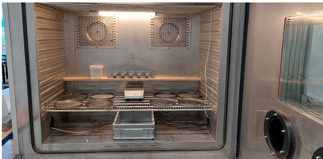
Fig. 1. Climate chamber for testing deicing performance according to SHRP H-205.1/2.
