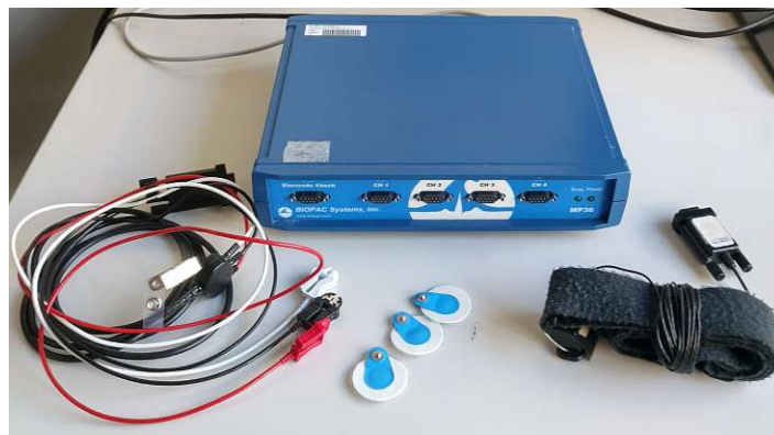
Figure 1-12: A photo of the BIOPAC System with ECG electrodes (left) and a respiration belt sensor (right)
