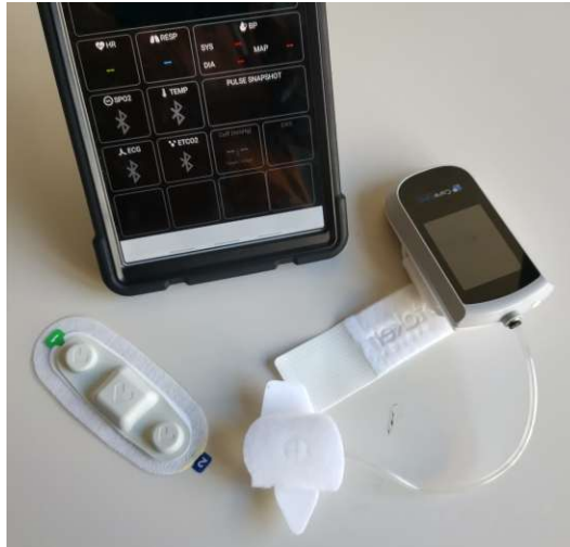
Figure 1-10: A photo of the Vitalstream™ finger cuff sensor(right) and the VIVALNK Bluetooth ECG monitor(left)
