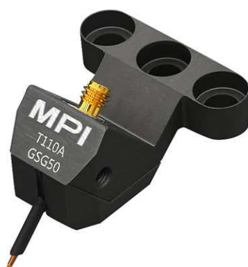
Figure 2.3: MPI T110A GSG50 probe, operates up to 110 GHz with a 1mm coaxial connector 1 .
