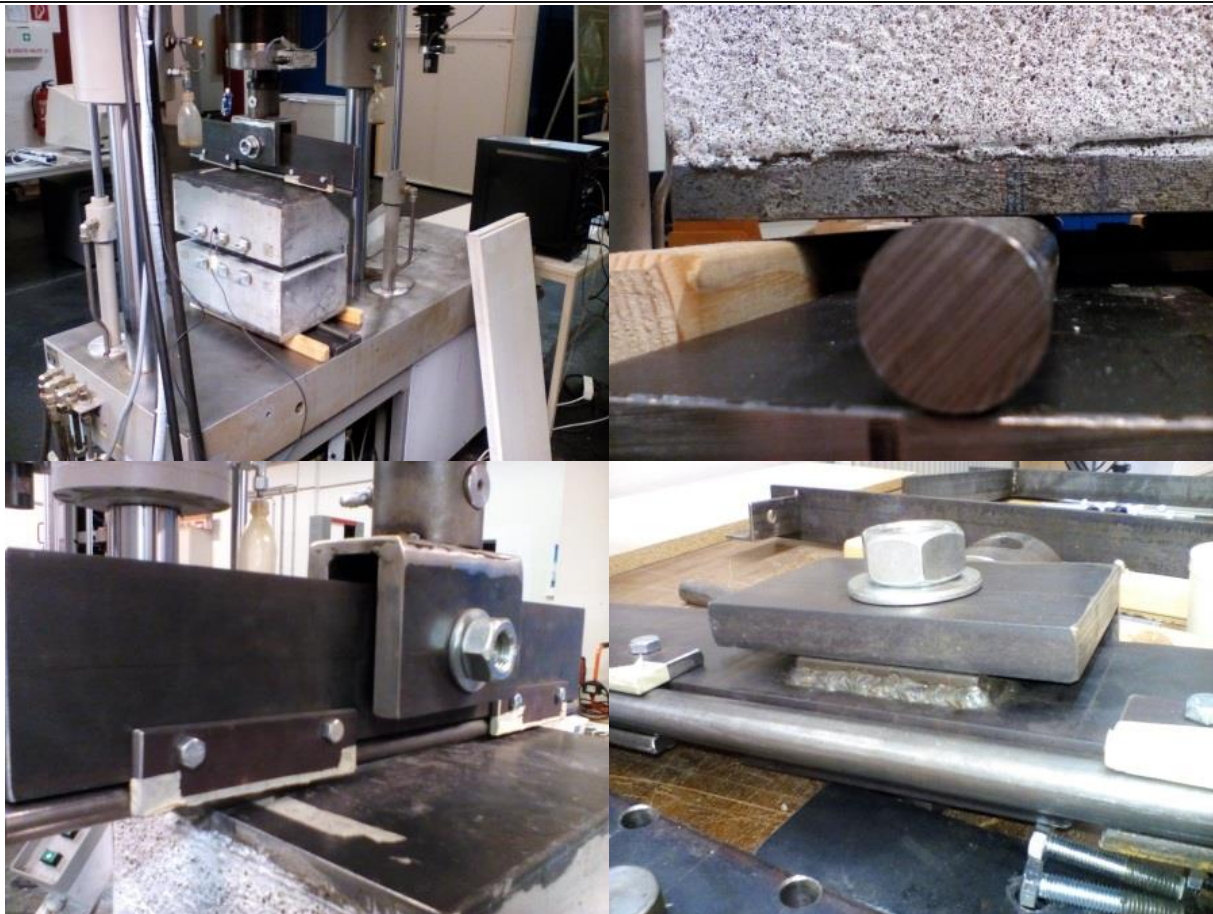
Fig. 8.15: Boundary-Conditions in Reality a)Model, b) bottom support; c,d)Loading plate
