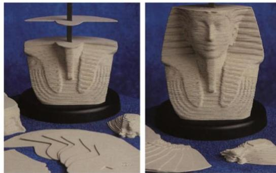
Figure 8: Principle of layer technology (Gebhardt & Hötter, 2016)
