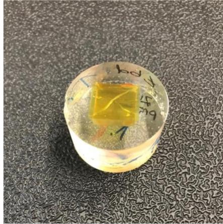
Figure 58: Embedded and polished sample
