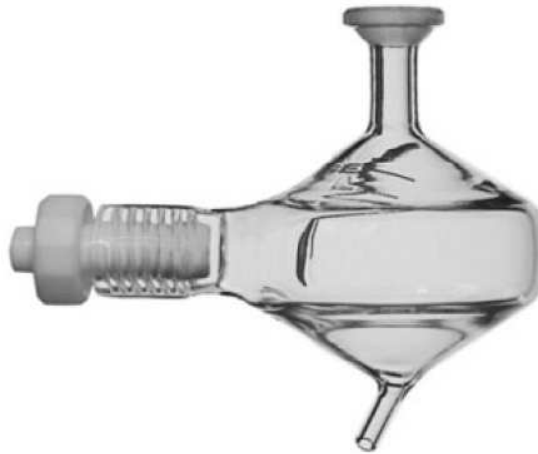
Figure 2.3: A cyclone spray chamber. The vapor enters from the side, the top exit leads to the torch, the bottom exit into the waste. [26]
