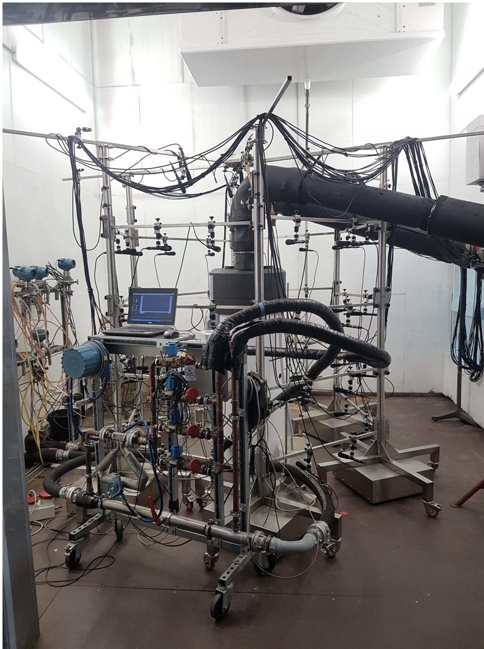
Figure 22: Photo of the setup used in the Point to Point procedure. The dome (with 55 microphones) is built around the indoor unit of a heat pump water heater, analyzed in the framework of the RRT4 (Round Robin Test 4) in Annex 51 of the IEA (International Energy Agency) HPT (Heat Pumping Technologies) programme [34]. The heat pump unit is obstructing the line of sight of microphones with with microphones on the opposite site leading to longer sound travel paths and wrong results. The air ducts for outside air in- and outlet are also obstructing the line of sight for microphones placed above them.
