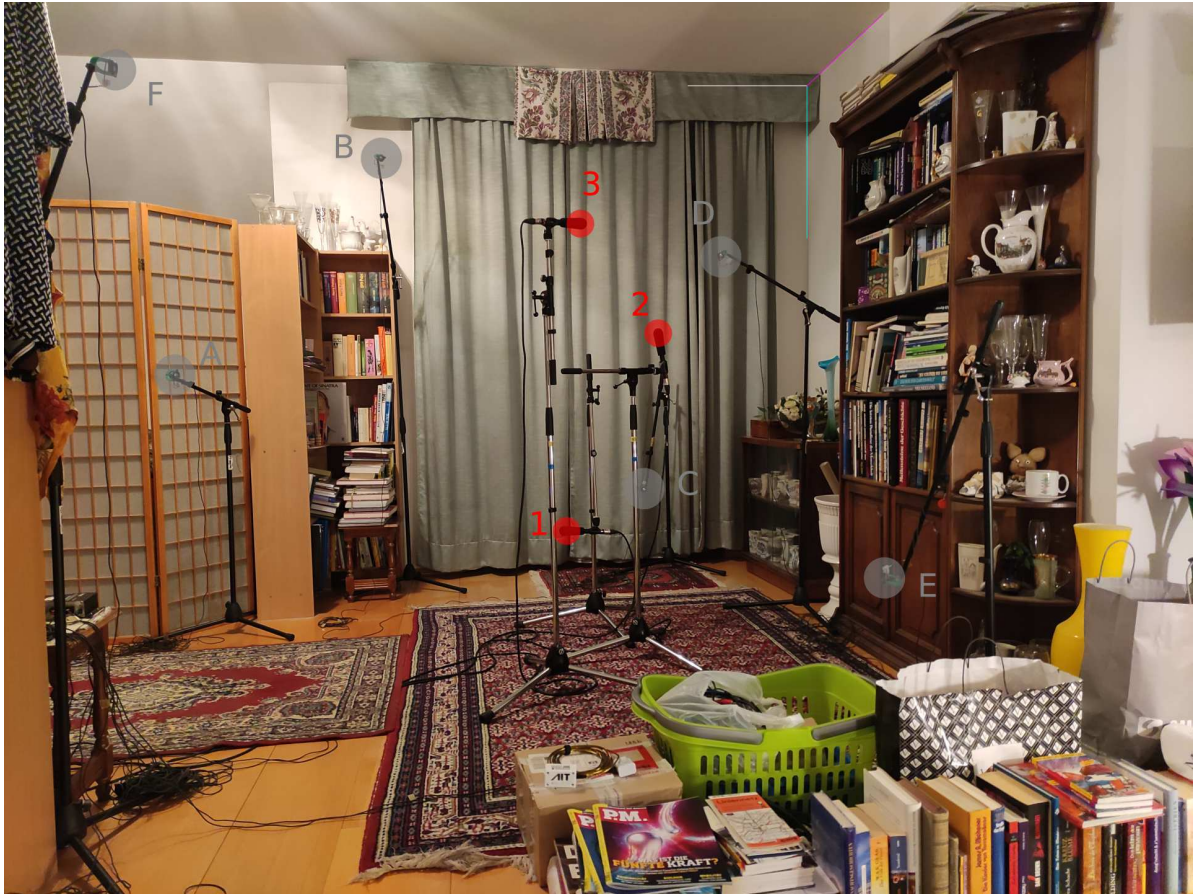
Figure 17: A photo of the experimental environment used for testing the localisation techniques. Carpets were laid out to prevent floor reflections. The coordinate system's origin and orientation can be seen in the top right room corner. Speakers were mounted on microphone stands with a self-designed 3D printed adapter. Their positions are emphasized with gray circles and labelled A through F . Three microphones were placed and their position manually determined with a laser distance meter. These reference positions are visualized in red and labeled 1, 2 and 3. The microphones' coordinates can be found in table 1 (also labelled as microphone 1, 2 and 3).
