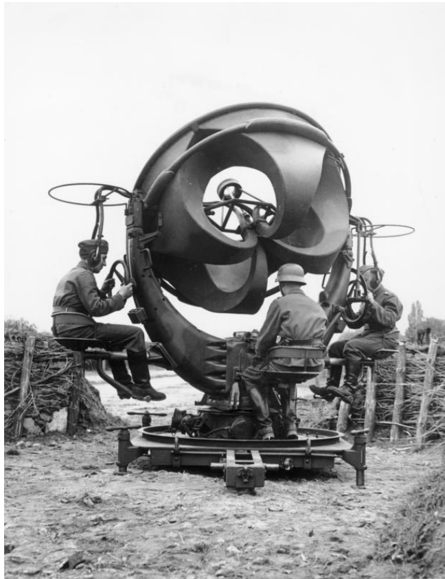
Figure 2: Sound location equipment "Horchgerät" in Germany, 1939. It consists of four acoustic horns, a horizontal pair and a vertical pair, connected by rubber tubes to stethoscope type earphones worn by the two technicians left and right. The stereo earphones enabled one technician to determine the horizontal direction and the other the elevation of the aircraft.
