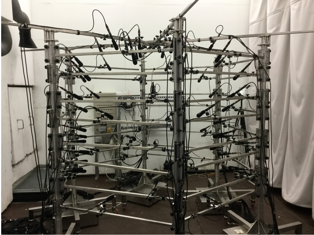
Figure 5: Photograph of the 64 channel setup in the dome arrangement with a six-sided symmetry. 61 microphones are used in this geometry. 8 arms are mounted to each of the six stands with one metal rod going to the middle. Microphones are positioned on each arm to maximize spread along the cylinder's surface area. Individual adjustments can be made if strong sound emission directivity is suspected. Two microphones are mounted on each top rod and one microphone is placed in the middle. In operation, the heat pump is placed in the middle of the microphone dome. To change hardware parts for different measurements, the arms need to be moved to gain access to the pump. Afterwards the arms need to be readjusted, which can alter the geometry and sound intensity at the microphone head.
