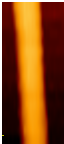
Figure 38: A force-map ( 0.8 \times 2 \mu\text{m} ) of a native fibril in PBS, before chemical modification (showing measured height). The size of an indentation-pixel is marked by the yellow rectangle.
