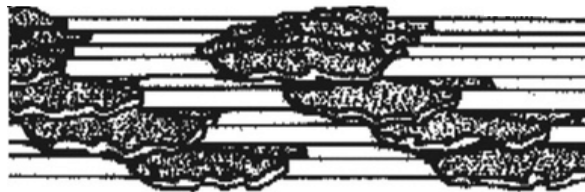
Figure 11: Schematic illustration of a mineralized fibril, crystallized between staggered TC struts [36]
