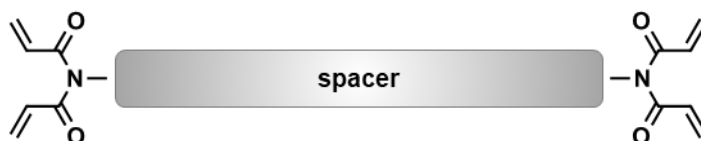
Figure 32: Schematic representation of a difunctional diacrylamide with different spacer units. 50
