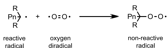
Figure 5: Mechanism of oxygen inhibition.
