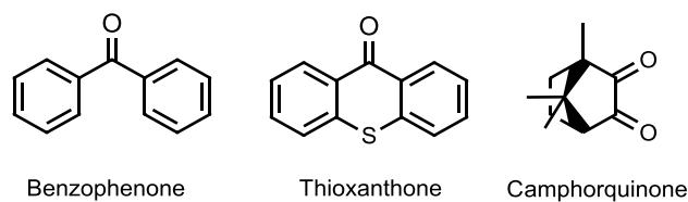
Figure 10: Industrial used Type II PIs: Benzophenone, thioxanthone and camphorquinone.
