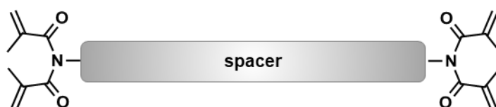
Figure 40: Schematic representation of a difunctional dimethacrylamide with exchangeable spacer unit.
