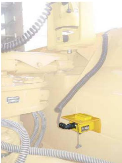
Abbildung 4-3: Querneigungssensor AS 400 von Trimble [60]
