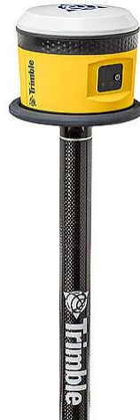
Abbildung 2-26: Roverstab von Trimble, "SPS585 Smart-Antenne" [63]
