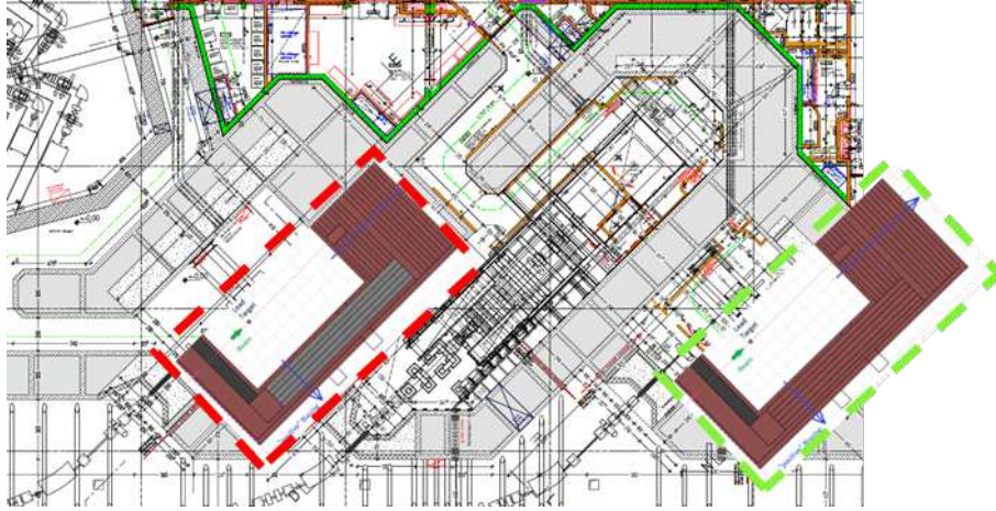
Figure 3.1: The original geometry of the irradiation room 1,2 and 3 of MedAustron compared to the generic cylindrically symmetrical geometry of IR1 and IR3 for lateral scoring. [1]
