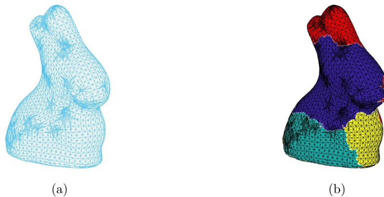
Figure 3.2: An example of segmentation of the object surface: (a) Triangular mesh model of the rabbit. (b) Result of the segmentation algorithm.
