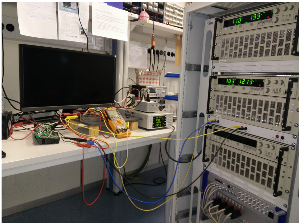
Figure 4.13: Setup in the lab. The power supply is located at the left, the adjustable load at the right, meters and other measurement instrumentation in the middle. [WLG+19]
