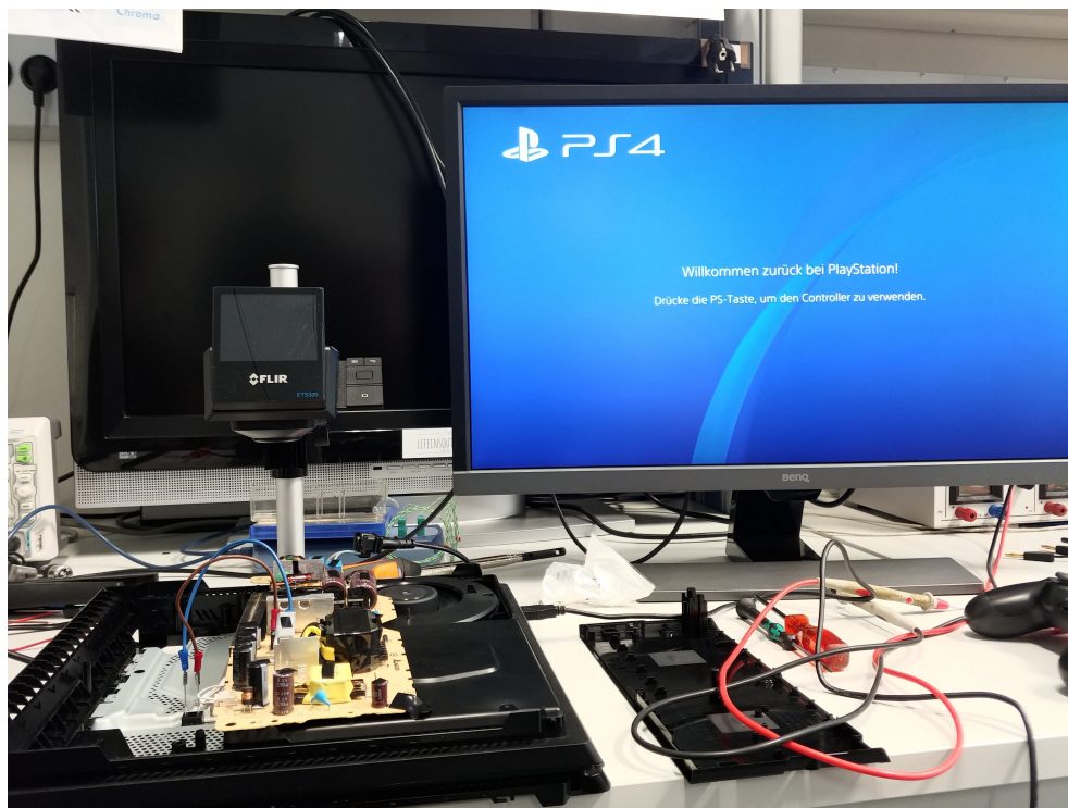
Figure 5.15: Setup for measuring the PS4 Pro with the thermal camera adapted for PCBs
