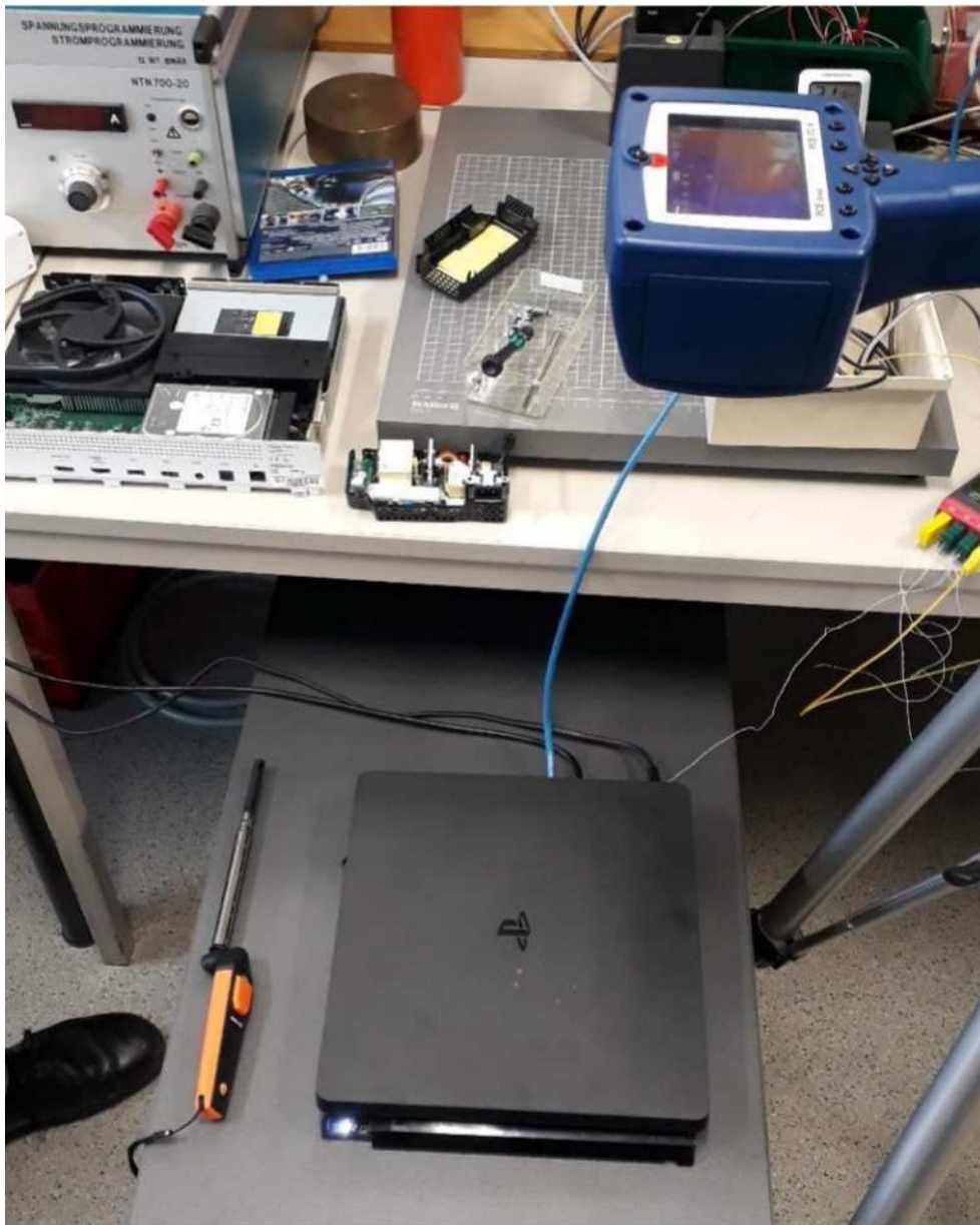
Figure 5.4: Setup for the thermal measurements with the infrared camera
