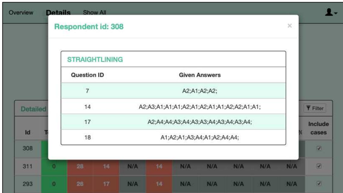
Figure 19. SQT straightlining view. The view highlights the questions, where a significant number of same answers in series per question matrix was given by the respondent.
