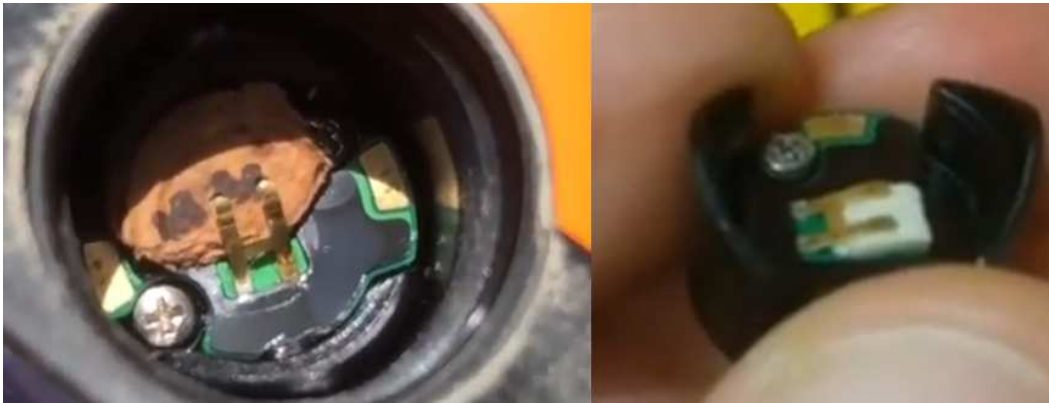
Figure 5.7: A piece of cork clamped in the spring contact to prevent the battery from losing contact.
