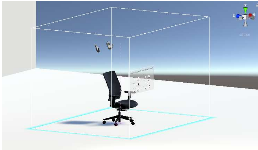
Figure 5.11: VR environment. LeapRig is shown as hands and a purple dotted line. The CameraRig is the turquoise rectangle on the floor together with the white lines forming a cube.
