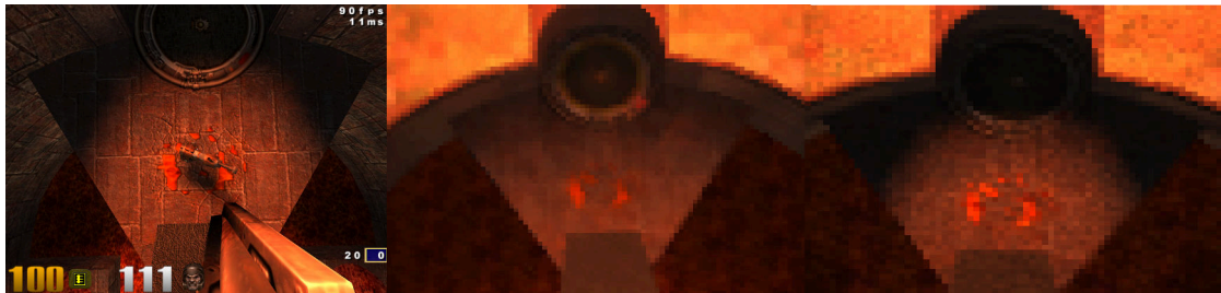
Figure 7.14: Left image shows the scene with the denoiser on, from a close distance. The middle image shows the result when the denoiser is on and the camera is further away from the object. The right image shows the accumulated image (no denoiser) from the same distance as the middle image. The shadows in the middle image are much lighter compared to the left and right image. The scene is taken from the map q3dm7.
