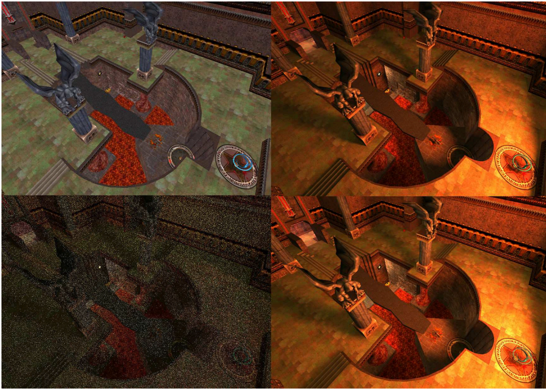
Figure 7.3: The top left image shows Quake III without light maps, which is equal to no illumination. Bottom left shows Quake III rendered with the ray tracer and one light per pixel. Top right is the ray traced result when using all 106 lights per pixel and no denoiser. The bottom right is the ray traced result with one light per pixel and a denoiser. The scene is take from the map q3dm7.
