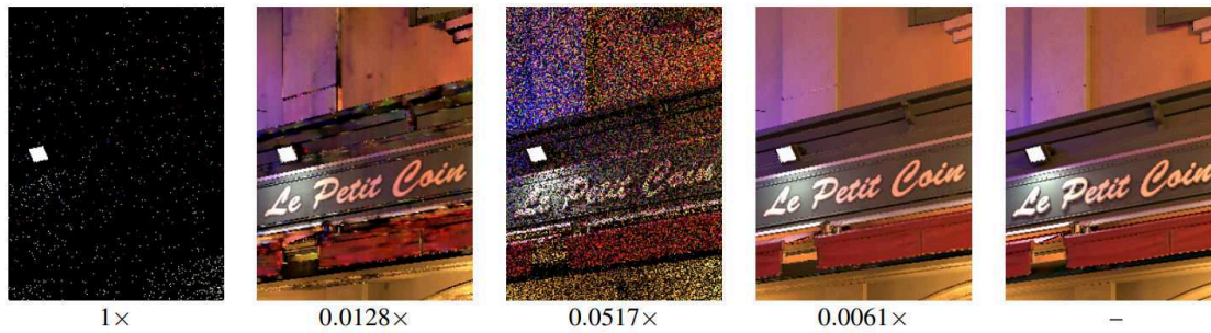
Figure 3.3: First two images are 1 spp with uniform sampled lights and denoised with SVGF [SSK + 17] over 5 frames. Next two images are 1 spp with BVH sampled lights and denoised with SVGF over 5 frames. The last image is the ground truth. [MPC19]
