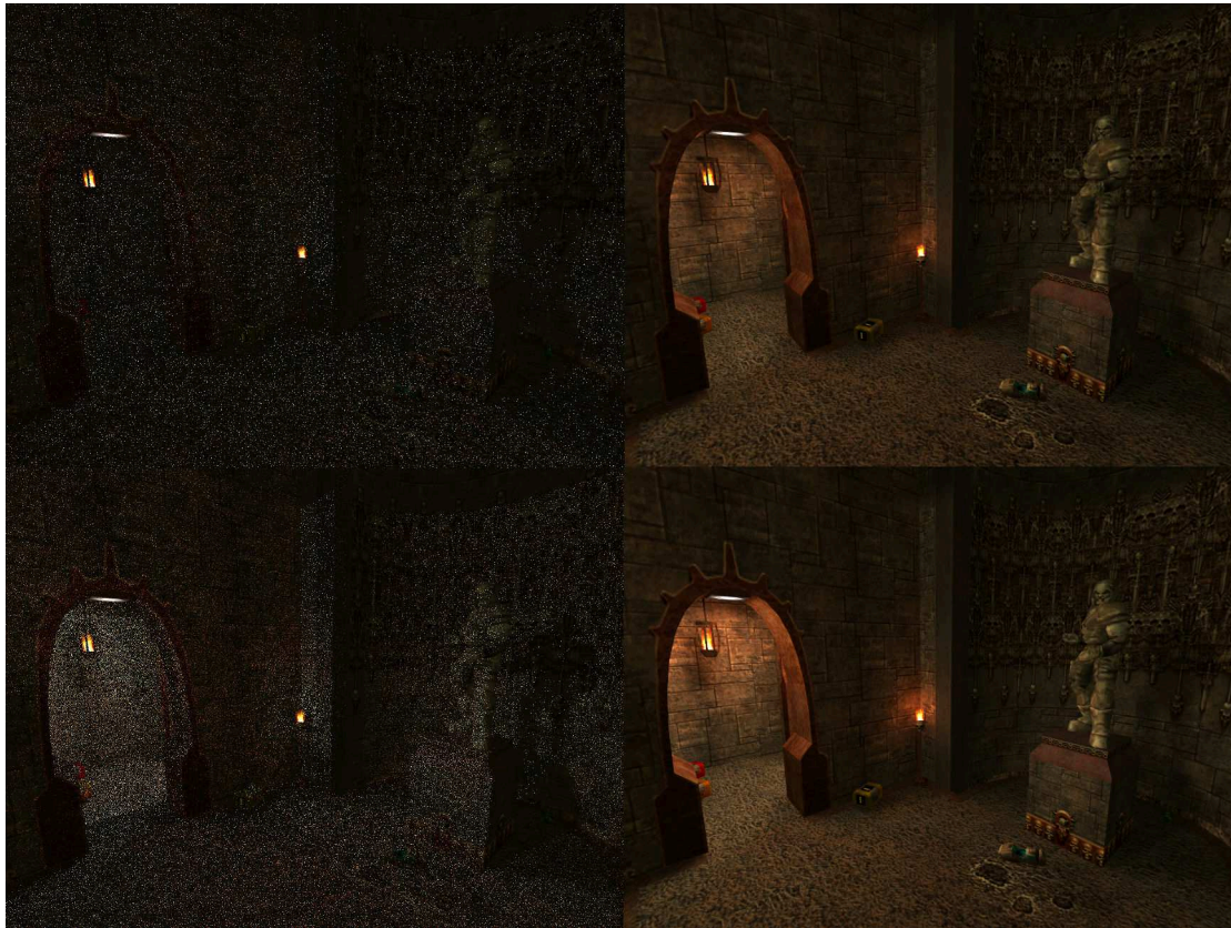
Figure 7.4: The top left image shows Quake III with the denoiser deactivated, one light per pixel and light culling off. Bottom left shows Quake III with the denoiser deactivated, one light per pixel and light culling on. Both images on the right show the images from the left processed by the denoiser. The scene is take from the map q3dm9.
