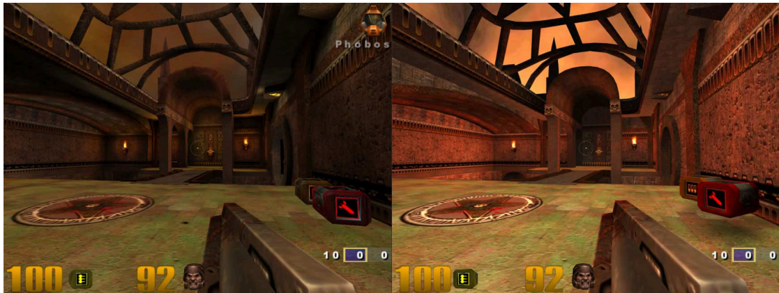
Figure 7.1: The left shows the original Quake III rasterizer. The right image is the result produced by our ray-tracing implementation. The scene is taken from the map q3dm2.
