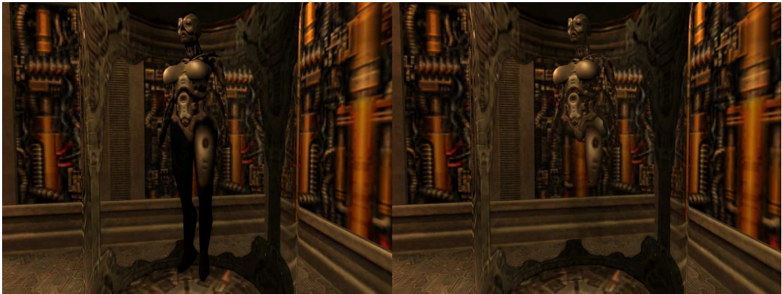
Figure 7.5: Glass tube with a semi-opaque model in between (from map q3dm0). Left image shows the scene with the secondary ray stage functionality for semi-opaque model deactivated.
