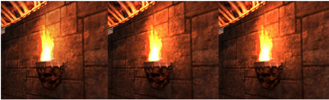
Figure 7.2: The left shows the ray-traced result without a denoiser and all 146 lights per pixel. The middle image shows the same but with TAA activated. The right image is the accumulation of 1500 frames with the same configuration as the left image. The scene is taken from the map q3dm4.
