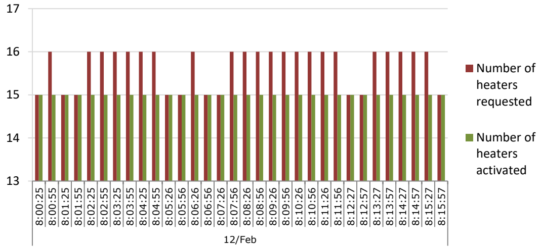
Figure 165. Number of heaters requested by BMS and corresponding number of heaters activated by load balancing unit from 08:00-08:15 o'clock. Date:12.02.2016
