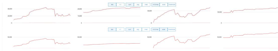
Figure 6.6: Different trend diagrams without (top) and with (bottom) uniform scaling applied. By using a common y-axis scaling, it becomes obvious that the value ranges of the two outmost projects on the left side are partly a way below the two on the right side, a fact that would not immediately be apparent if every diagram uses its own axis scaling.
