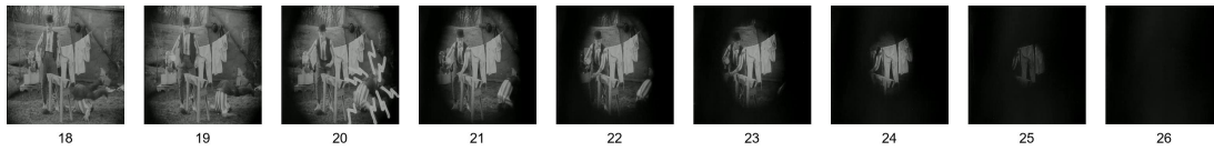
(a) Iris In: The frame content moves into a circle which gradually decreases. The transition ends with a monochromatic frame.
