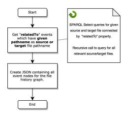
Figure 6.10: Process of creating JSON Nodes of a file-history by service *FileHistoryService*.
