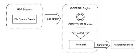
Figure 6.4: Process of C-SPARQL engine to handle RDF streams
