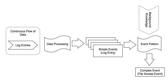
Figure 6.3: Complex Event Processing: flow from Log Entry to Complex Event
