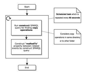
Figure 6.9: Flow of scheduler task in service *FileHistoryService*.
