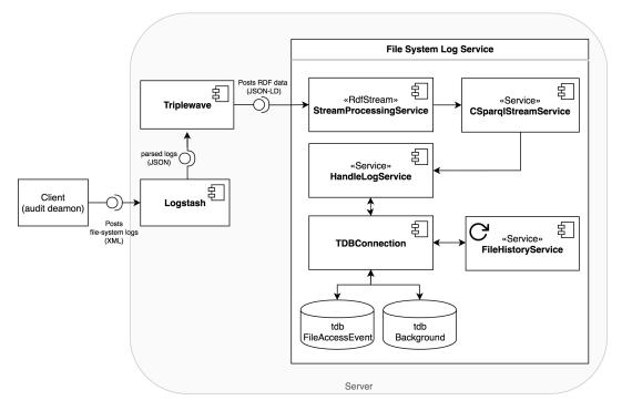
Figure 6.1: Architecture Diagram of prototype
