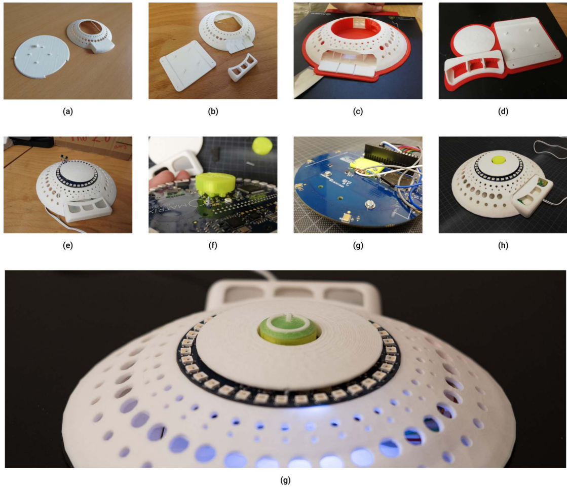
Figure 5.14: Development of the probe casing.
