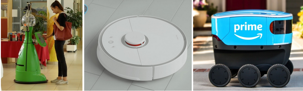
Figure 1.1: Examples of robots that provide services in real environments. The robots have robust navigation skills to provide services such as guiding a person, displaying information, cleaning a floor, delivering packages. Left: Werner from EU STRANDS 1 project, Middle: Roborock5 2 from Roborock Technology Co., Ltd, Right: Scout 3 from Amazon.
