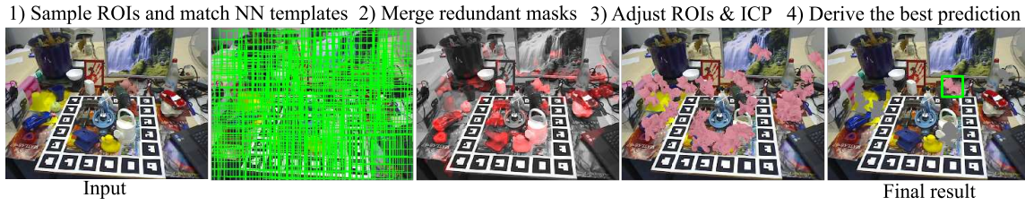
Figure 5.3: The overview of the pose estimation process with an input depth image. Color images are used only for visualization.
